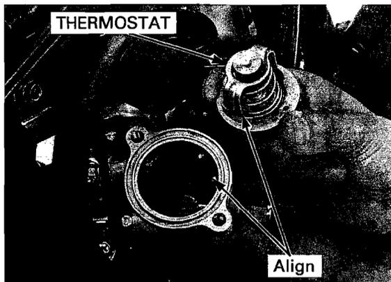
Install a new O-ring into the thermostat housing groove.
