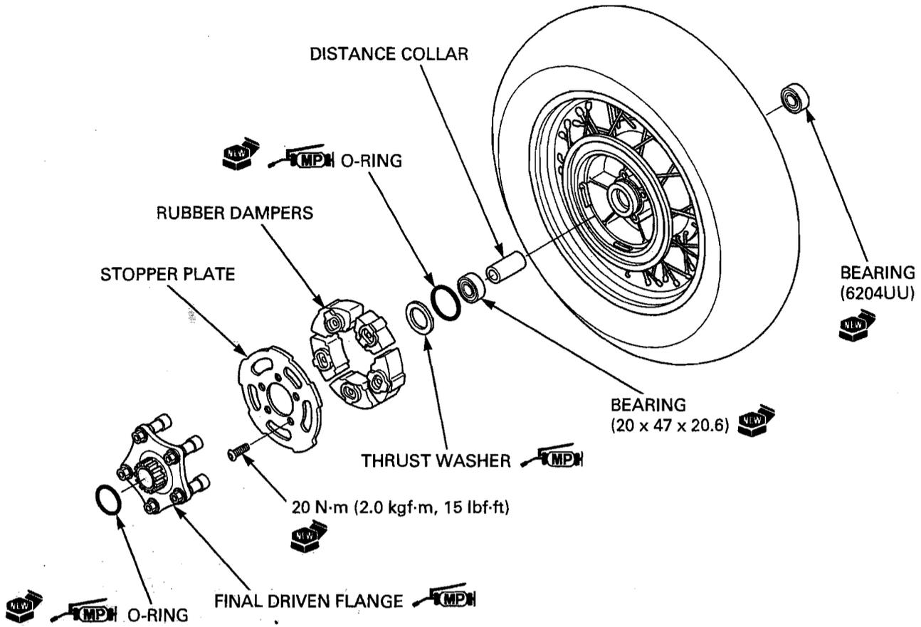
Drive in a new right bearing squarely with the marked side facing up until it is fully seated.
