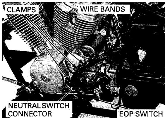
Connect the ignition pulse generator 2P (Red) connector.
