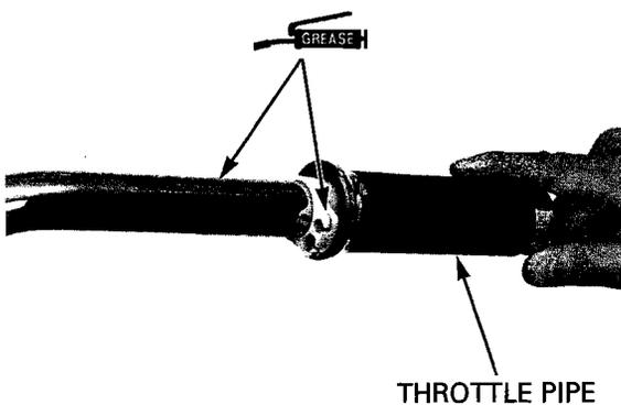
Connect the throttle cables to the throttle pipe flange.
