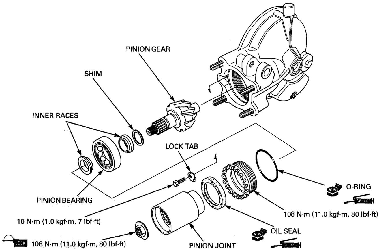
Drive the pinion gear assembly into the gear case using the special tool.
