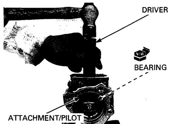
Press a new bearing into the bearing holder with the marked side facing up until it is fully seated and make sure it rotates freely after installation.
