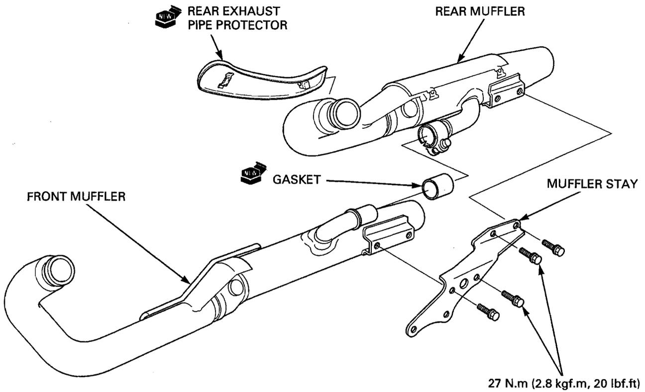
Install a new gasket onto the front muffler joint pipe.
