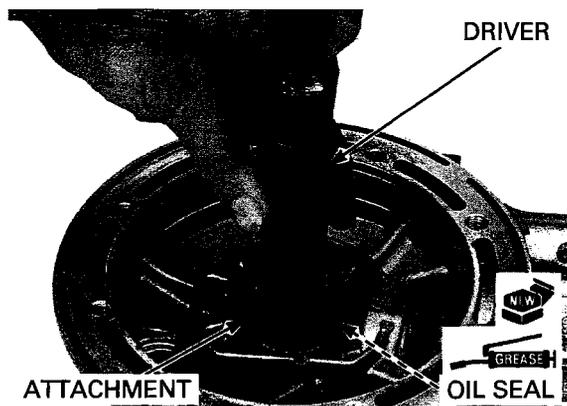
Drive a new ring gear case bearing into the gear case with the marked side facing inside until it is fully seated using the special tools.
