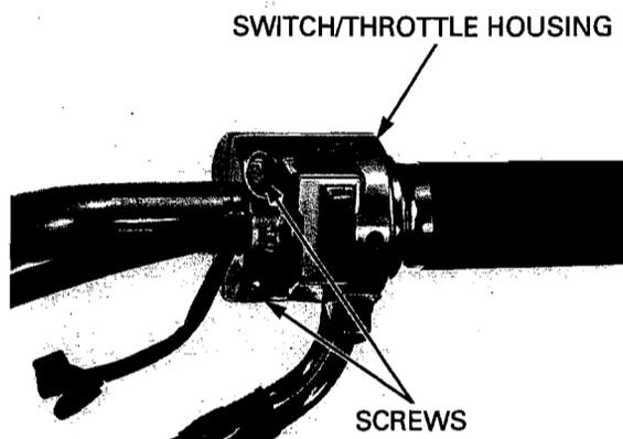
Disconnect the throttle cables from the throttle pipe and remove the throttle grip from the right handlebar.
