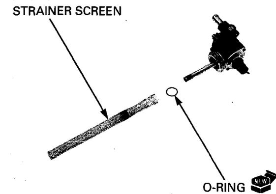
Install the fuel valve into the fuel tank.
