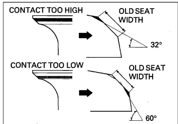
Using a 45° cutter, remove any roughness or irregularities from the seat.
