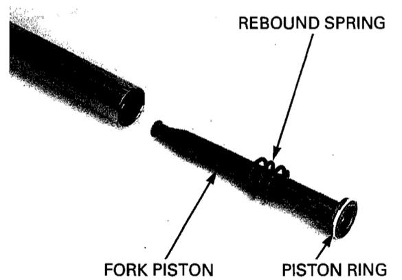
Install the oil lock piece and spring to the fork piston end.
