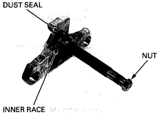
Apply specified grease (page 1-19) to a new dust seal lip and install it onto the steering stem. Press a new lower bearing inner race using a special tool and hydraulic press.
