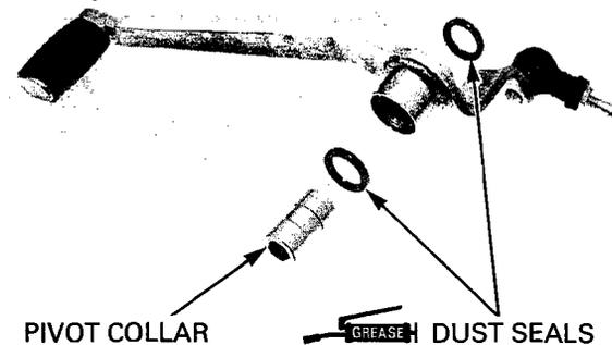
Install the gearshift pedal, washer and pivot bolt.
