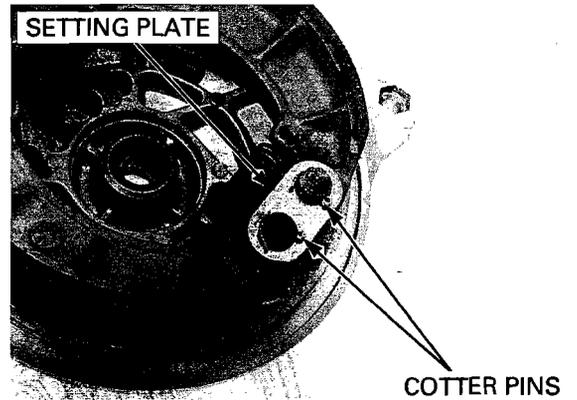
Remove the brake shoes and springs.
