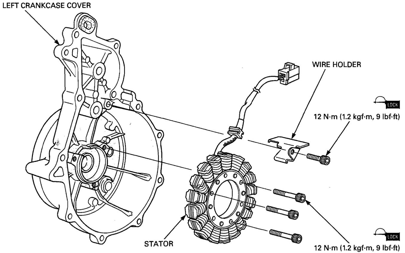
Install the stator to the left crankcase cover. Clean and apply a locking agent to the bolt threads (page 1-19). Install and tighten the stator socket bolts to the specified torque.
