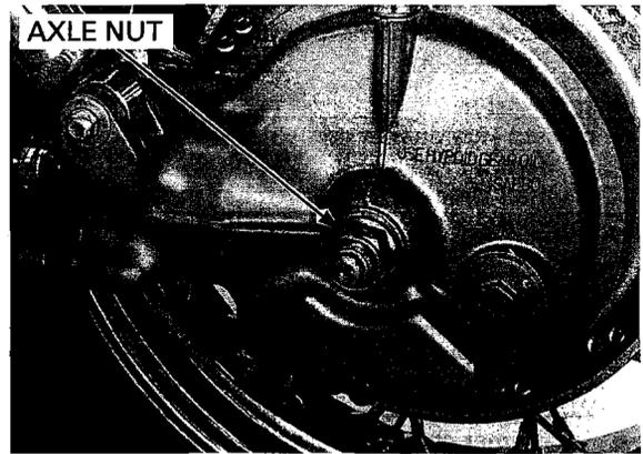
Remove the adjusting nut, joint pin and spring.
