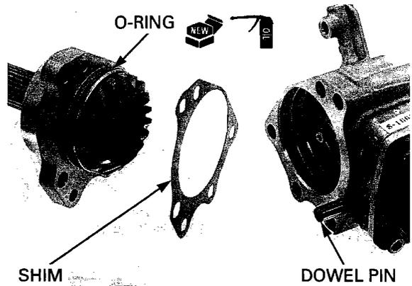
Install the drive gear assembly into the gear case.
