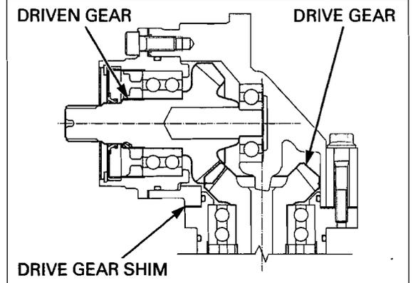
**OUTPUT DRIVE GEAR SHIM REPLACEMENT**
