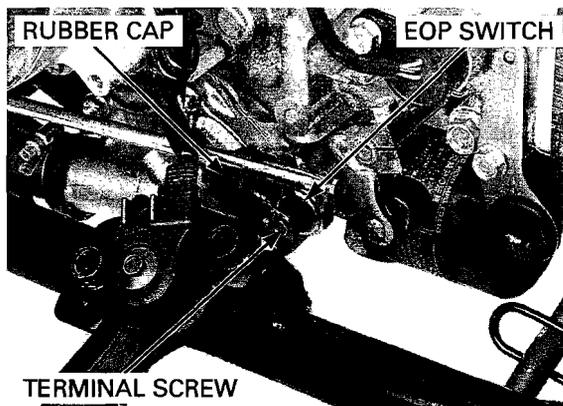
Remove the EOP switch and connect an oil pressure gauge attachment and gauge to the EOP switch hole.
