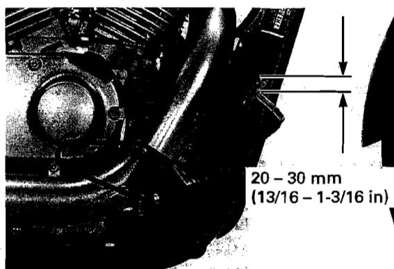
*Make sure the cut-out on the adjusting nut is seated on the joint pin.*
