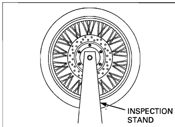
To balance the wheel, install a new balance weight on the lightest side of the spoke, on the side opposite the chalk marks. Add just enough weight so the wheel will no longer stop in the same position when it is spun.
