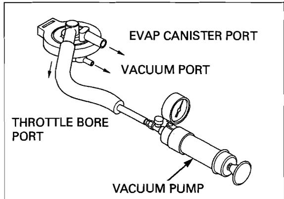
Remove the vacuum pump and connect it to the vacuum port.
