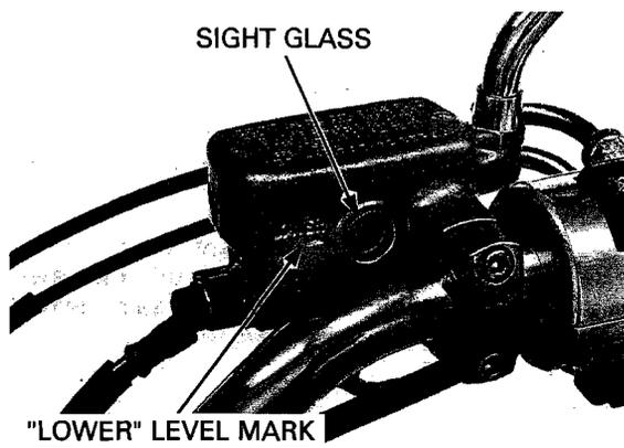
If the fluid level is near the "LOWER" level mark, remove the screws, reservoir cap, set plate and diaphragm.
