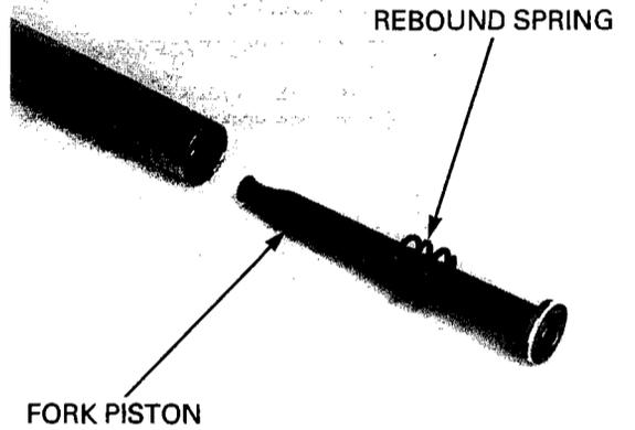
Using quick successive motions, pull the fork tube out of the fork slider.
