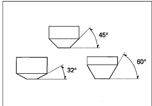
If the contact area is too high on the valve, the seat must be lowered using a 32° flat cutter.
