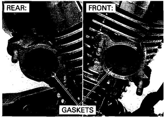
Remove the exhaust pipe joint collars and flanges.
