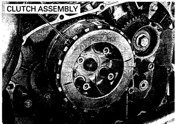
Install the end clutch disc into the shallow slots of the clutch outer.
