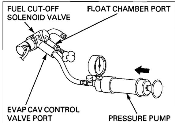
Connect the 12 V battery to the fuel cut-off solenoid valve 2P connector terminals.
