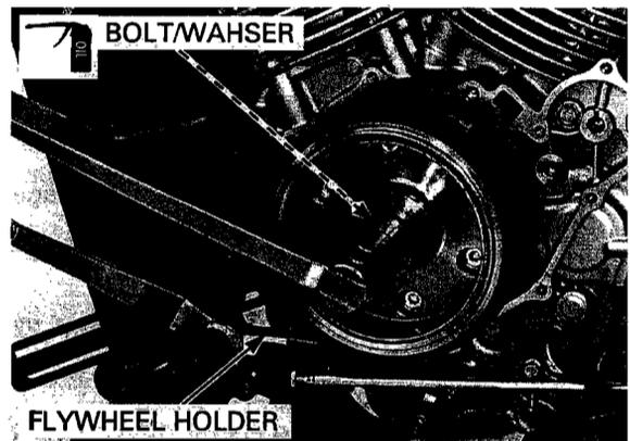
*The flywheel bolt has left hand threads.*
