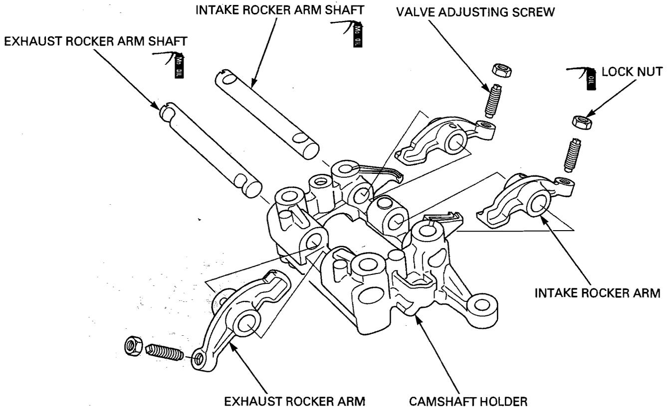
*When disassembling the valve adjusting lock nut and adjusting screw.*
