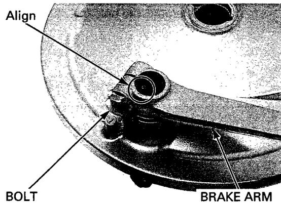
Apply 0.5 – 1.0 g of grease to the brake shoe-to-anchor pin sliding surface.
