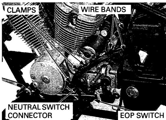
Remove the pinch bolt and gearshift arm.
