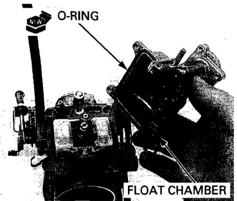
Install the float chamber and tighten the float chamber screws to the specified torque.
