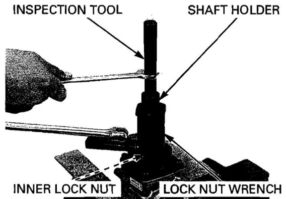
Remove the bearing outer race lock nut using a special tool.
