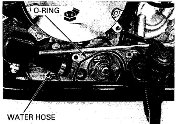
Align the bolt holes in the pump and crankcase, then install the water pump cover with the bolts and a new sealing washer.
