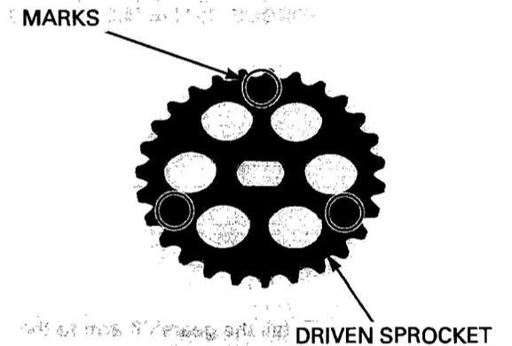
Apply locking agent to the oil pump driven sprocket bolt threads and install the washer and bolt.
