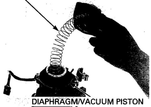
*Be careful not to damage the diaphragm.* Turn the jet needle holder counterclockwise using a screwdriver while pressing it in and release the holder flange from the vacuum piston.
