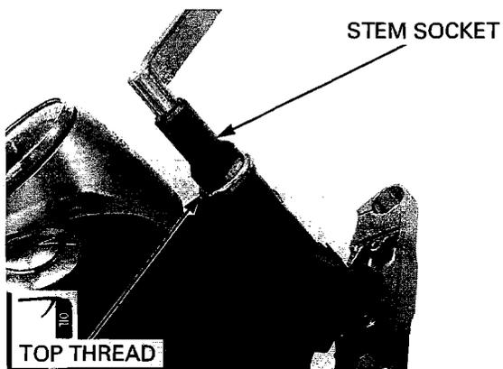
Turn the steering stem left and right, lock-to-lock five times to seat the bearings.
