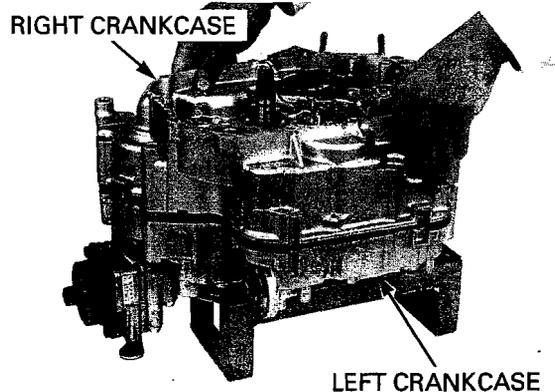
Turn the shift drum until the position as shown. Install the right crankcase bolts with the washer. Tighten the 8 mm bolts in a crisscross pattern in several steps.
