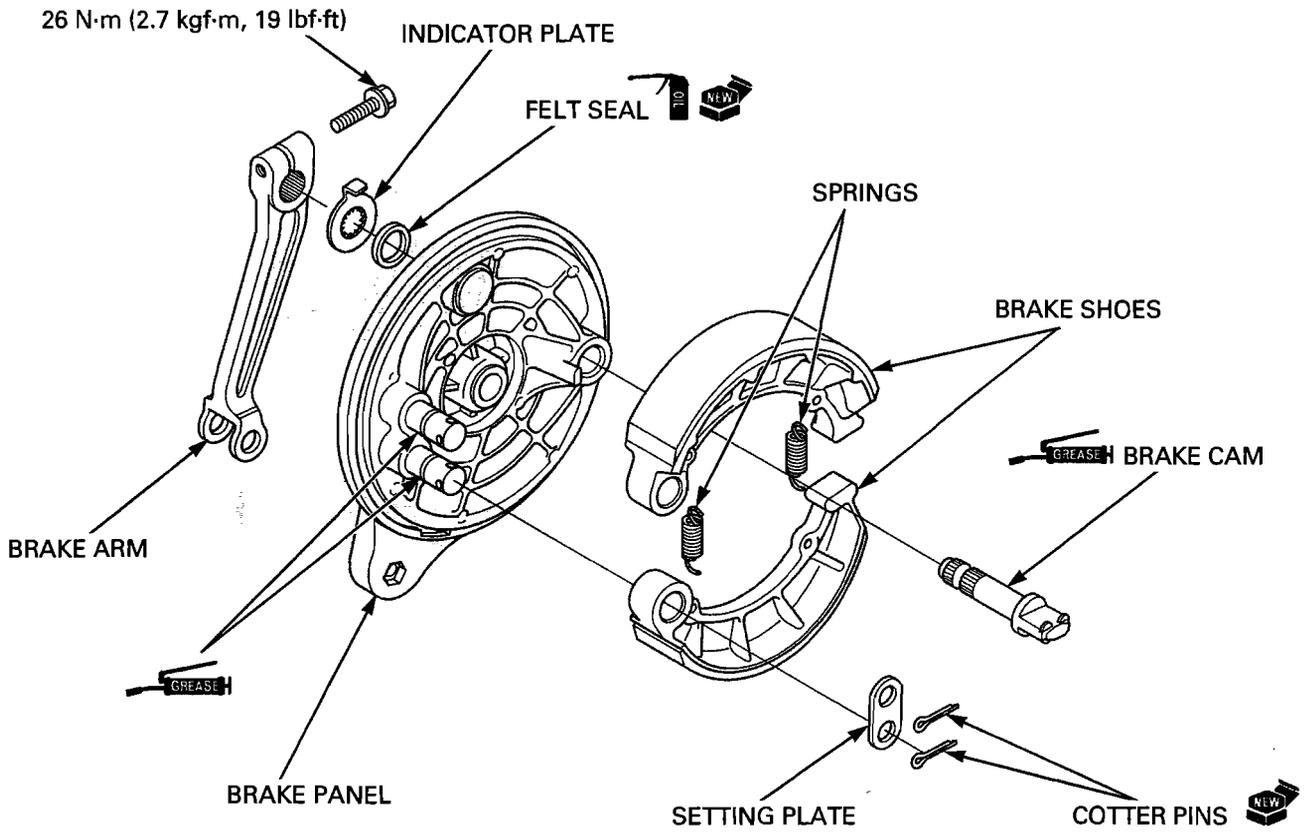
Apply 0.5 – 1.0 g of grease to the brake cam sliding surface.
