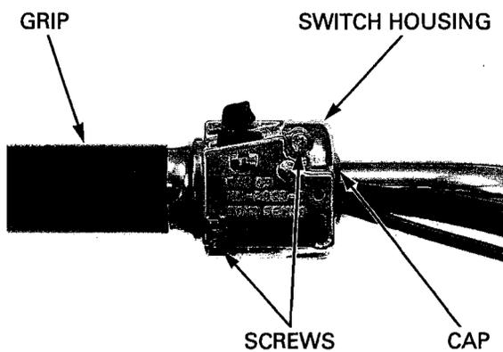
Disconnect the front brake light switch wire connectors from the switch.
