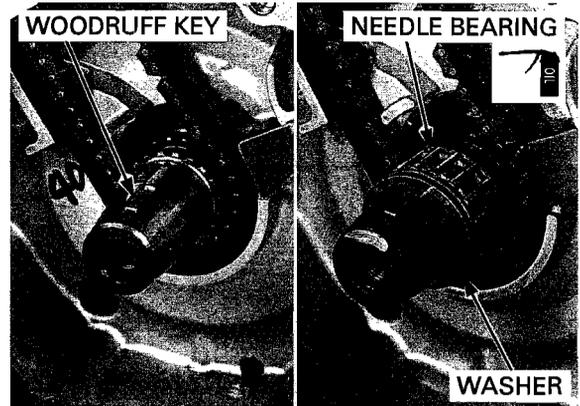
Wipe any oil off the mating surface of the flywheel. Install the flywheel to the crankshaft, aligning the key groove of the flywheel with the woodruff key on the crankshaft.
