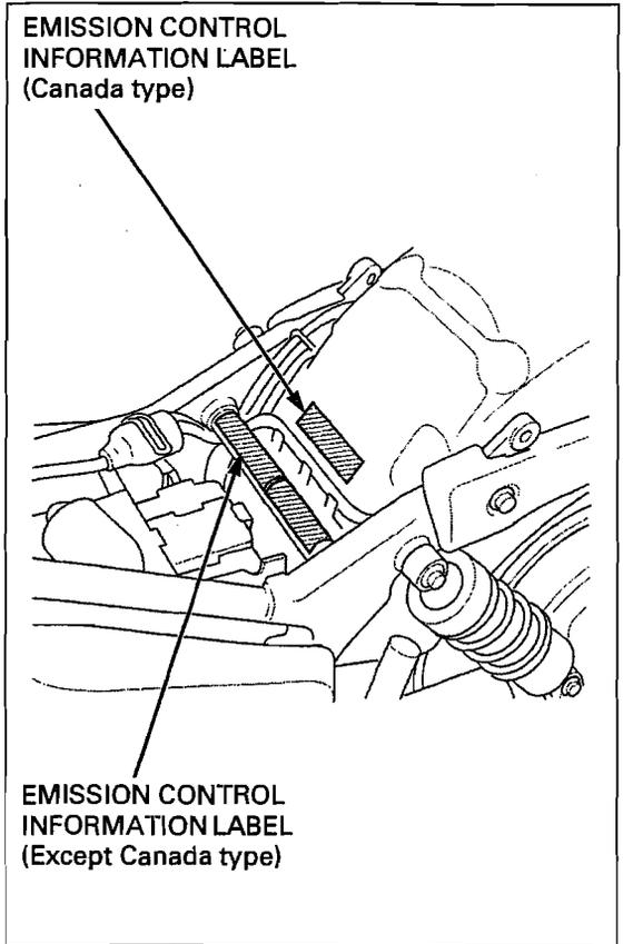
The Emission Control Information Label (After '07) is located on the left side of the frame down tube.
