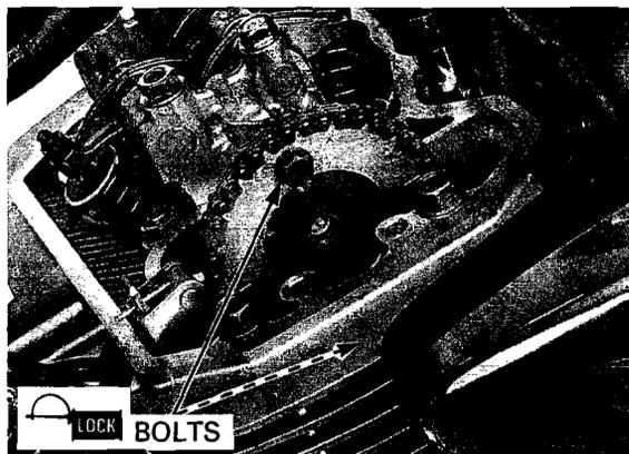
Remove an O.D. 2 mm pin while holding cam chain tensioner wedge A and pushing down the wedge B.
