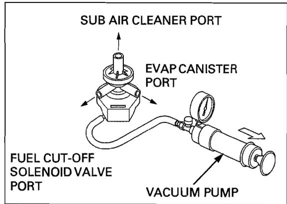
Remove the vacuum pump and connect it to the sub air cleaner port.
