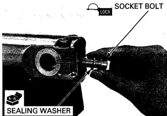
*If the fork piston turns with the fork center socket bolt, temporarily install the fork spring, spring seat, spacer and fork cap.*
