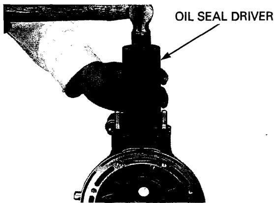
Apply grease to a new oil seal lips.
