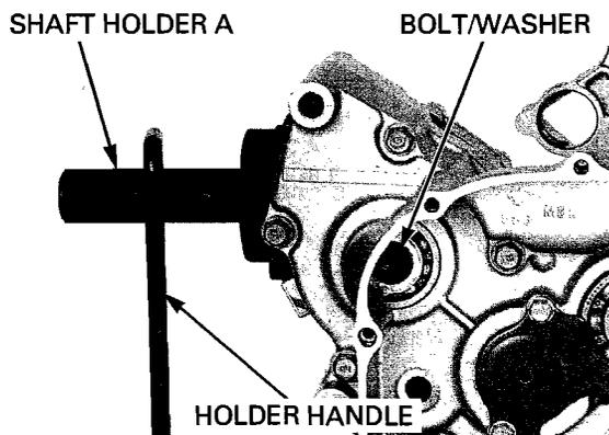
Remove the bolts and bearing setting plate.
