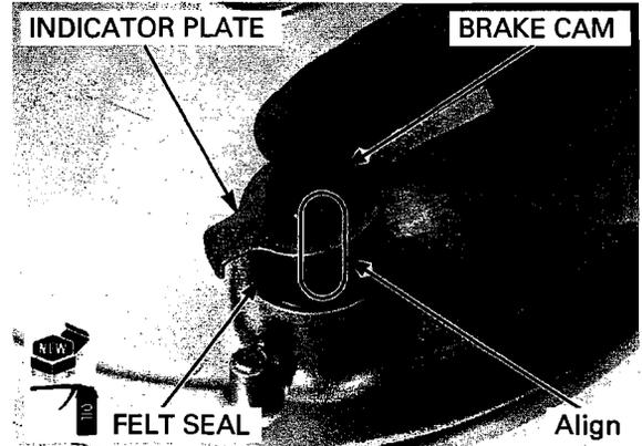
Install the brake arm aligning the punch marks of the arm and the brake cam.
