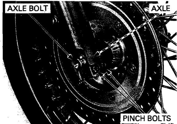
With the front brake applied, pump the forks up and down several times to seat the axle and check brake operation.
