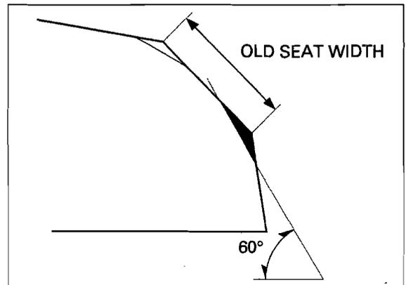
Using a 45° seat cutter, cut the seat to the proper width. Make sure that all pitting and irregularities are removed.
