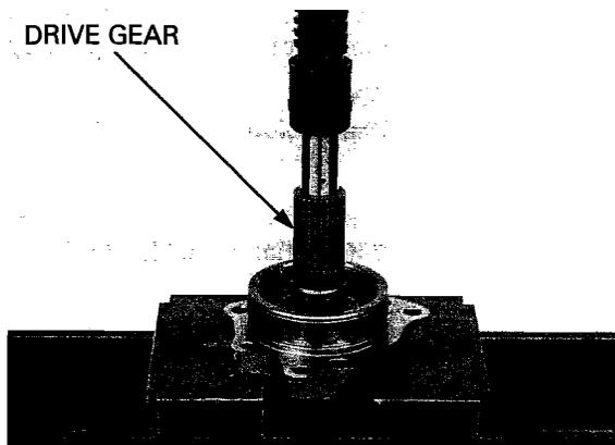
Press the drive gear bearing out of the bearing holder using the special tools and a hydraulic press.
