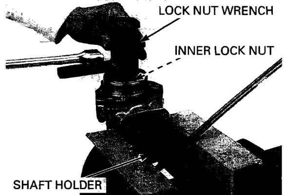
Remove the bearing outer race lock nut using a special tool.
