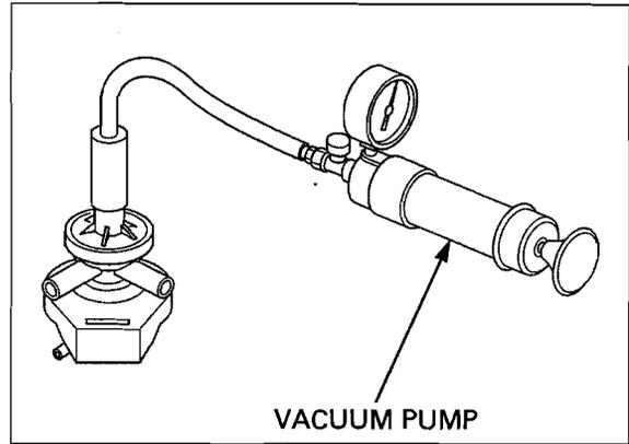
Remove the vacuum pump and reconnect it to the vacuum port.
