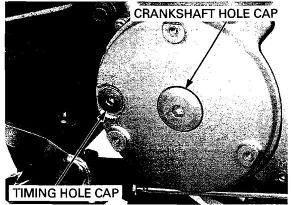
Turn the crankshaft counterclockwise and align the "RT" mark (front cylinder: "FT" mark) with the index notch on the left crankcase cover. Make sure the piston is at TDC (Top Dead Center) on the exhaust stroke so the piston is at TDC on the compression stroke when removing the camshaft holder.
