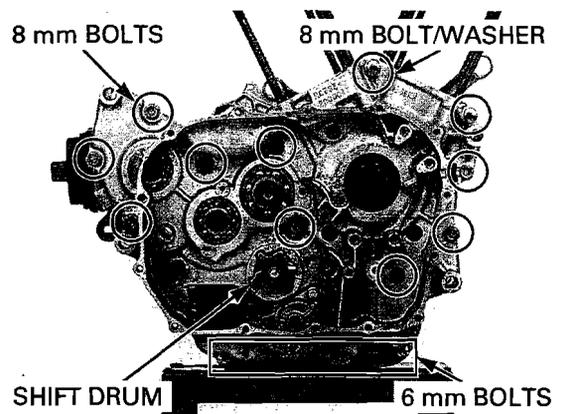
Place the crankcase with the left crankcase down and remove the right crankcase.
