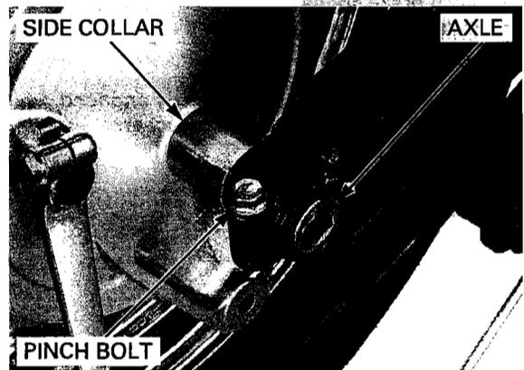
Remove the left side collar from the ring gear.
