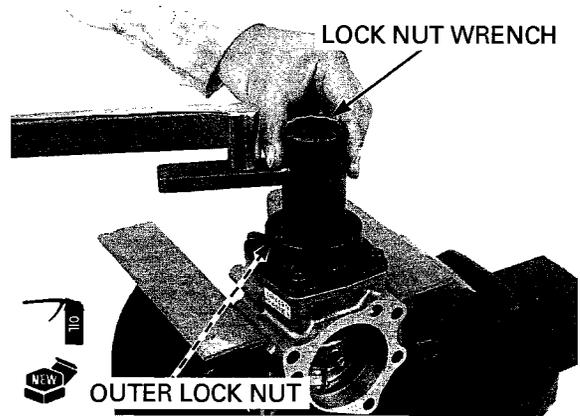
Apply engine oil to the threads and seating surface of a new inner race lock nut.
