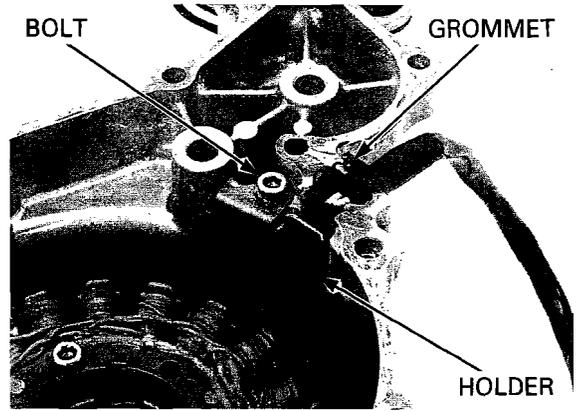
Remove the bolts and stator from the left crankcase cover.
