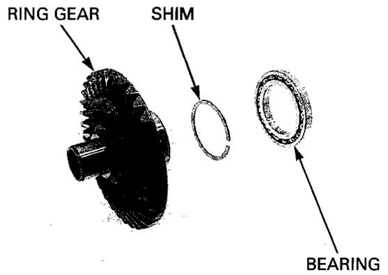
Press the ring gear bearing into the cover with the marked side facing inside until it is fully seated.
