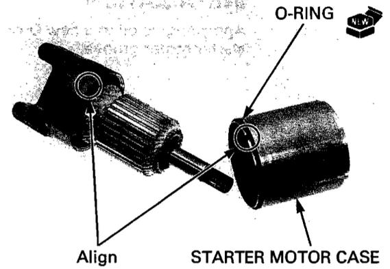
Install a new O-ring to the starter motor case. Install the front cover to the starter motor case.
