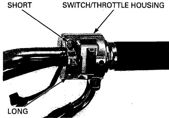
*Install the holder with its "UP" mark facing up.*
