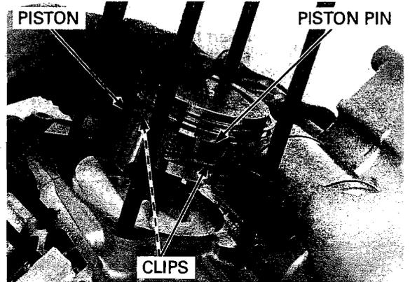
*Do not damage the piston ring by spreading the ends too far.*
