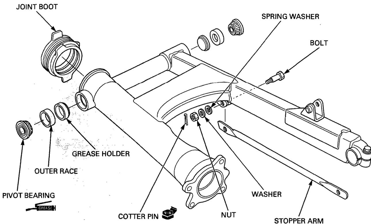
Apply 1.0 – 1.5 g of specified grease (page 1-19) to the needle rollers and dust seal lips of each bearing. Install the pivot bearings into the swingarm pivots.
