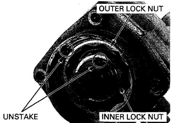
Hold the driven gear shaft and remove the bearing inner race lock nut using the special tools.
