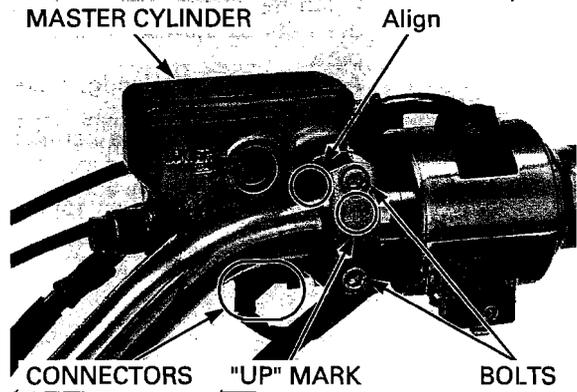
*Set the housing cap flange into the housing groove.*
