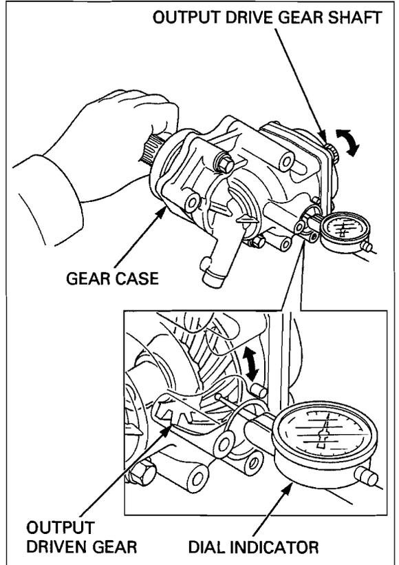
If the backlash is excessive, replace the output drive gear shim with a thinner one. If the backlash is too small, replace the output drive gear shim with a thicker one.
