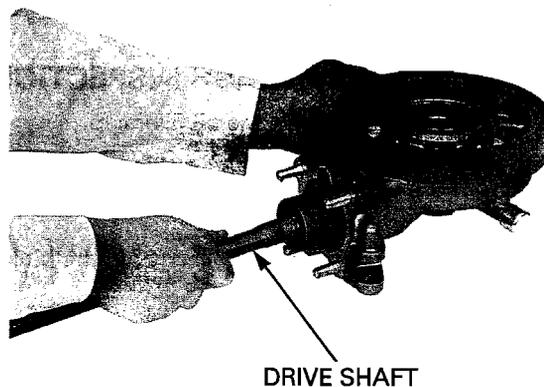
Remove the spring, oil seal and stopper ring from the drive shaft.
