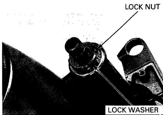
Loosen the steering top thread using the special tool.
