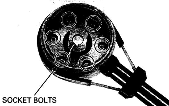
Remove the starter clutch outer/one-way clutch from the flywheel.
