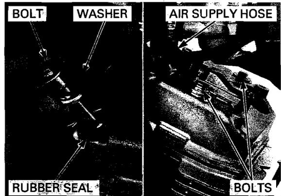
Install the front left over head cover and tighten the socket bolts to the specified torque.
