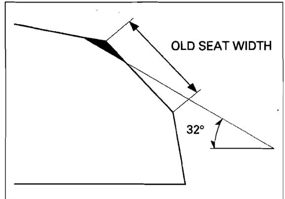
Using a 60° cutter, remove the bottom 1/4 of the old seat.
