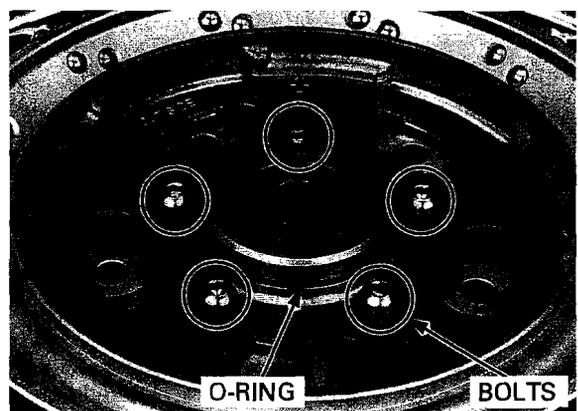
Align the arrow on the stopper plate between the projections on the wheel hub by turning the stopper plate and remove the stopper plate.
