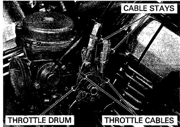
Connect the carburetor to the insulator while aligning its lug with the insulator groove. Tighten the insulator band screw securely.
