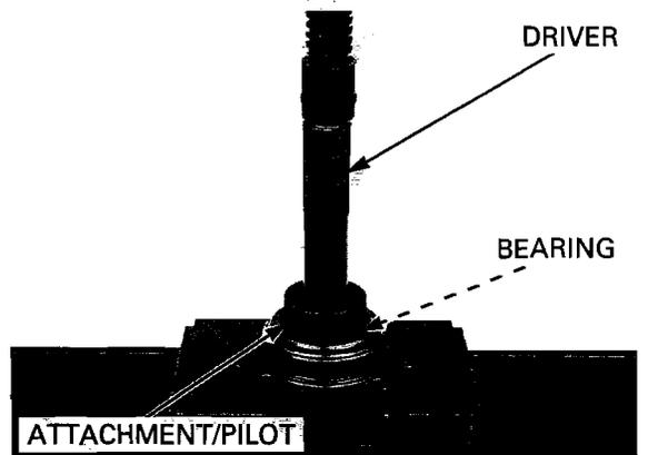
Remove the driven gear case bearing using the special tools.
