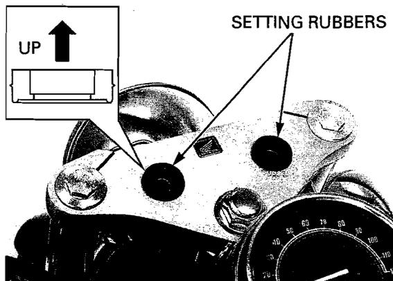
Install the handlebar lower holders, washers and nuts onto the top bridge.
