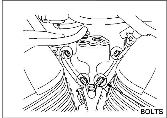
Install the choke cable stay and bolts.
