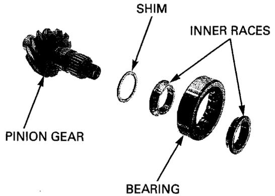
Drive the bearing with the marked side facing up.
