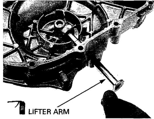
Install the return spring by inserting its short end into the clutch lifter arm groove.
