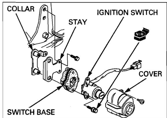
*The ignition switch mounting bolt heads are broken by tighten them to the specified torque.*
