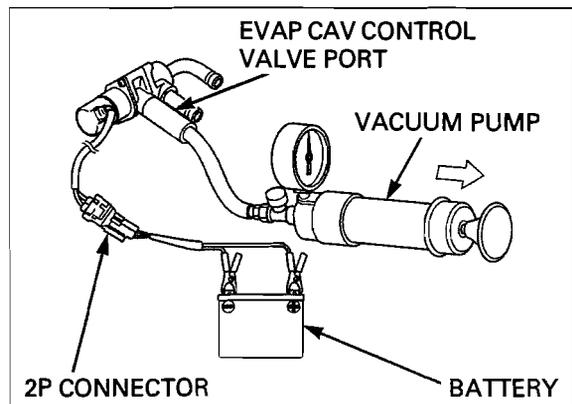
Remove the pressure pump and connect it to the vacuum port.
