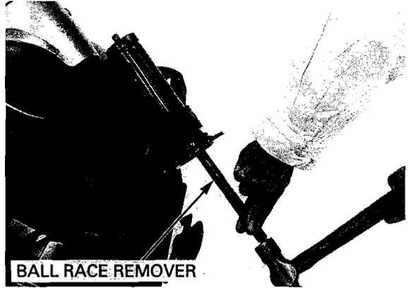
Remove the lower bearing outer race using the special tool and suitable shaft.
