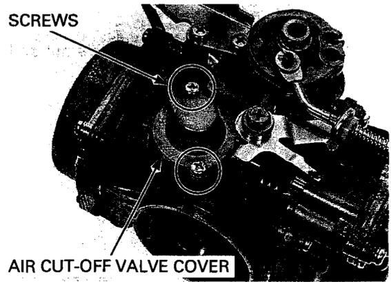
Remove the air cut-off valve cover, spring and air cut-off valve/diaphragm from the carburetor body.
