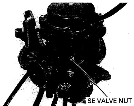
Pull the SE valve knob all the way out to fully open position and recheck for smooth operation of the SE valve knob.
