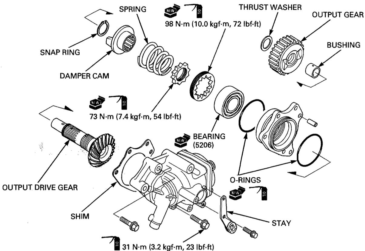
Press a new bearing into the bearing holder with the marked side facing up until it is fully seated.
