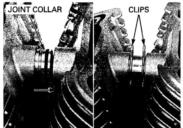
*Front cylinder only:* Install a new O-ring into the water hose joint groove.
