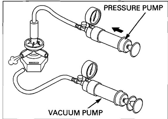
*Damage to the EVAP CAV control valve may result from use of a high pressure air source. Use a hand-operated air pump only.*
