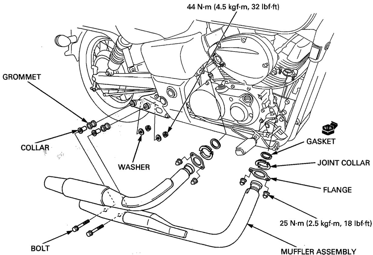
If the exhaust pipe joint stud bolts are loose, tighten them. Be sure to verify the distance from the top of the stud to the cylinder head as shown.
