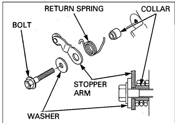
Hold the stopper arm with the screwdriver, and tighten the bolt securely as shown.
