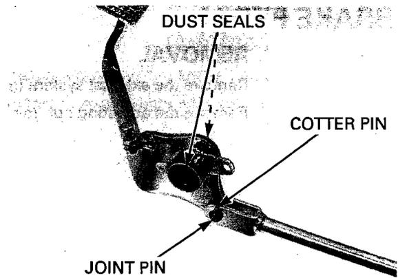
Remove the cotter pins and joint pins.
