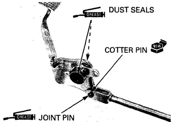
Apply grease to the brake pedal pivot sliding surface.
