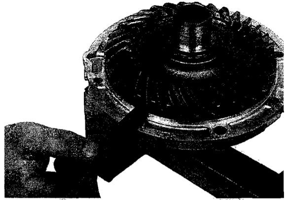
*Be sure to wear heavy gloves when handling the heated gear case.*
