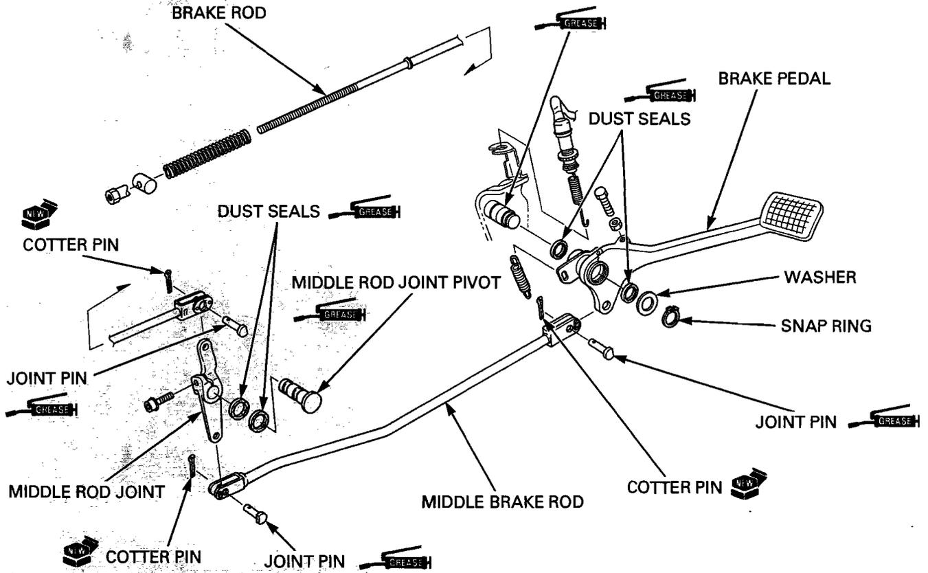
Apply grease to the joint pins.
