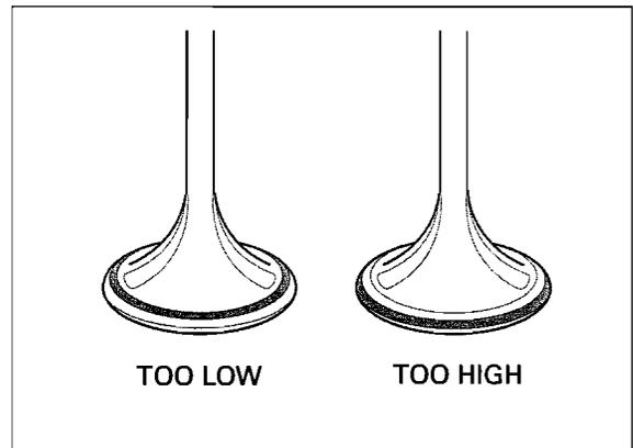
Inspect the width of the valve seat.
