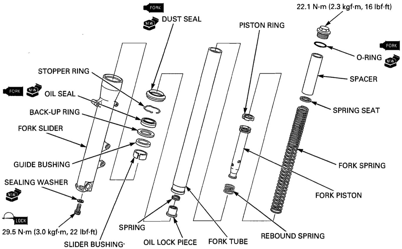
Do not open the bushing slit more than necessary.
