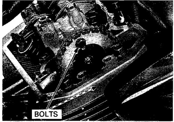
*Attach a piece of wire to the cam chain to prevent it from falling into the crankcase.*
