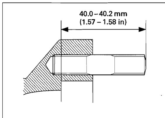
Install the flanges and exhaust pipe joint collars.
