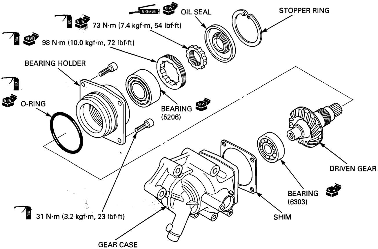
Drive a new bearing into the gear case with the marked side facing up until it is fully seated.
