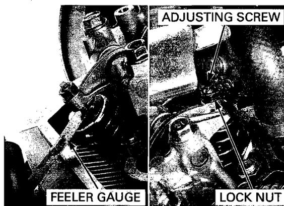
Adjust by loosening the valve adjusting screw lock nut and turning the adjusting screw until there is a slight drag on the feeler gauge.
