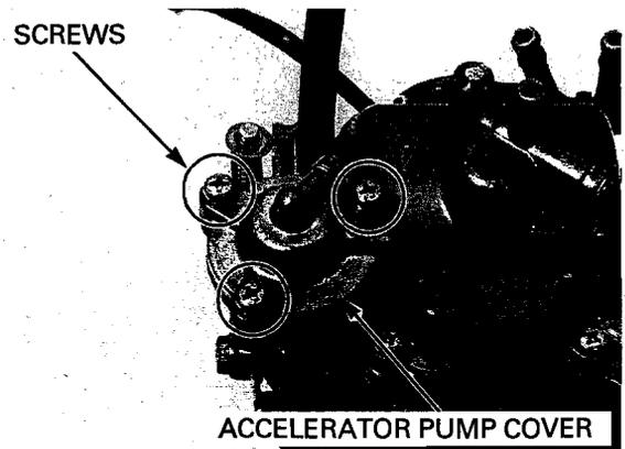
Remove the accelerator pump cover, spring and diaphragm/rod from the carburetor body.
