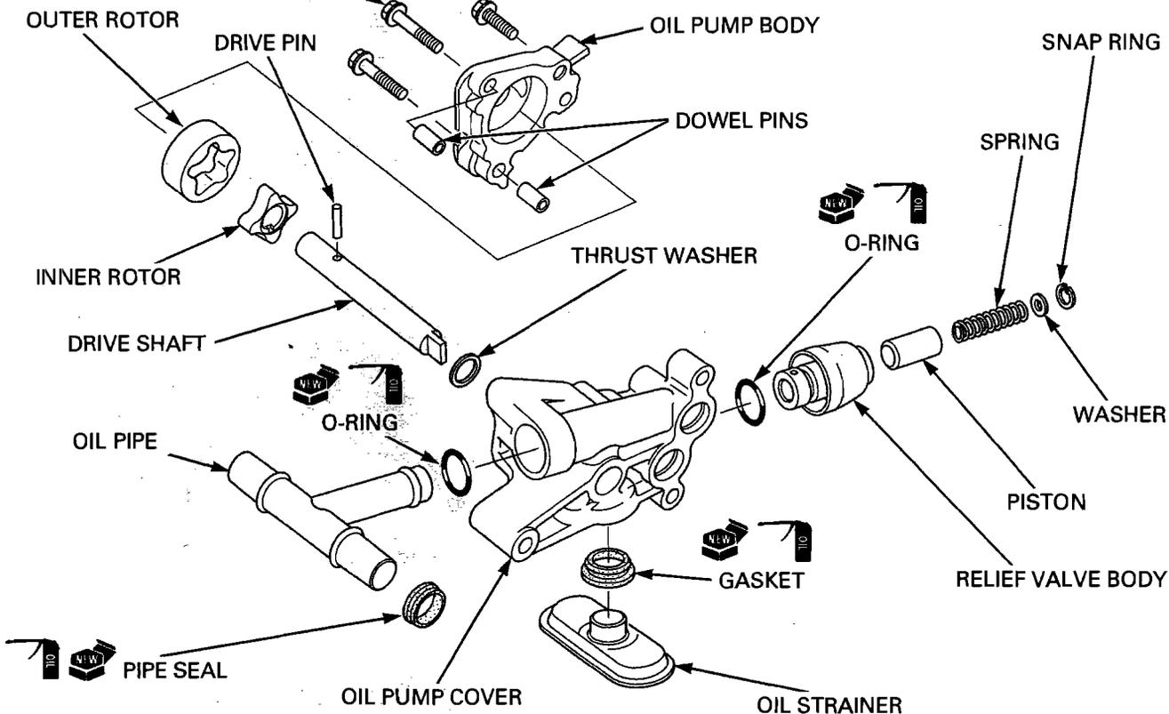
Install the outer and inner rotors to the pump body.
