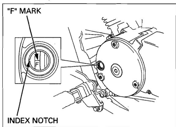
Coat a new O-ring with engine oil and install it into the timing hole cap groove. Apply grease to the threads of the timing hole cap. Install the timing hole cap and tighten it to the specified torque.
