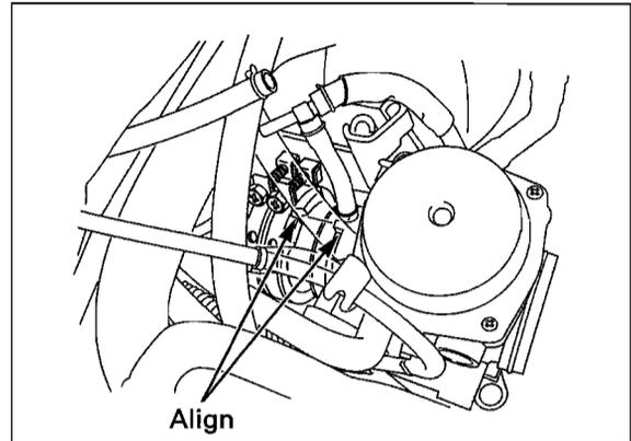
*Except california type:* Connect the air vent hose to the clamp.
