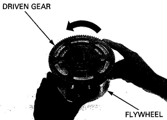
Remove the socket bolts while holding the flywheel using a special tool.
