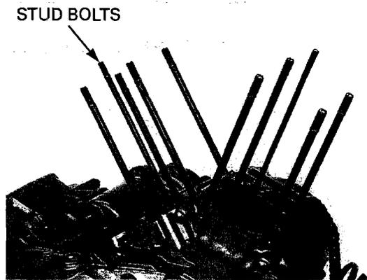
Apply engine oil to the lower threads of a new stud bolt and install it.
