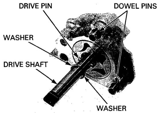
Install the pump cover on the pump body.
