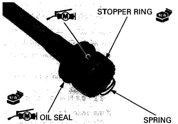
Apply 2 g or more of molybdenum disulfide grease to the pinion joint splines.
