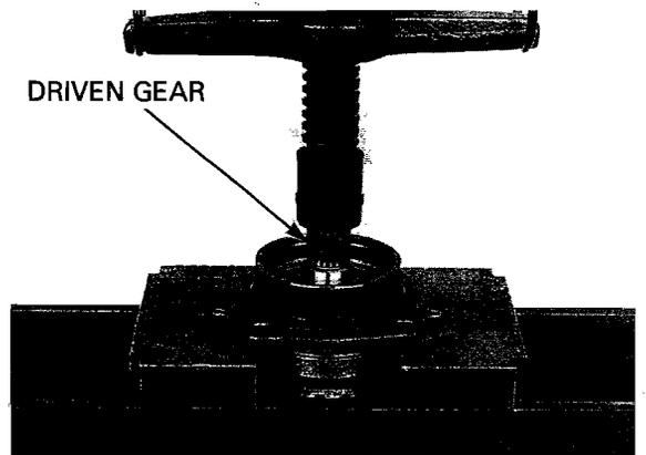
Press the driven gear bearing out of the bearing holder using the special tools and a hydraulic press.
