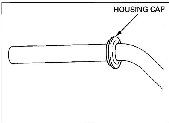
Clean the inside surface of the handlebar grip and the outside surface of the handlebar and throttle pipe. Apply Pro Honda Handgrip Cement or equivalent to the inside surface of the handlebar grip and to the outside surface of the handlebar and throttle pipe. Wait 3 - 5 minutes and install the grip.
