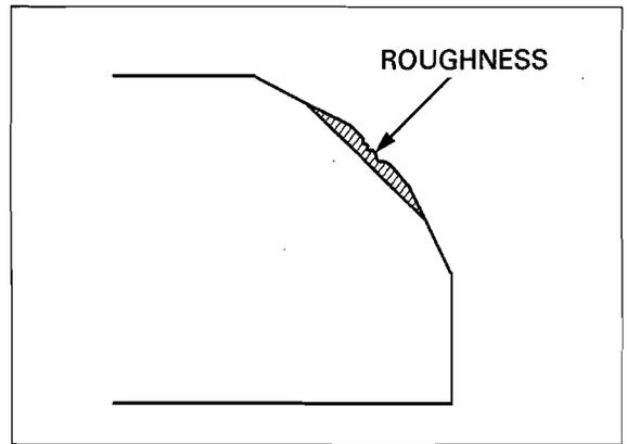
Using a 32° cutter, remove the top 1/4 of the existing valve seat material.
