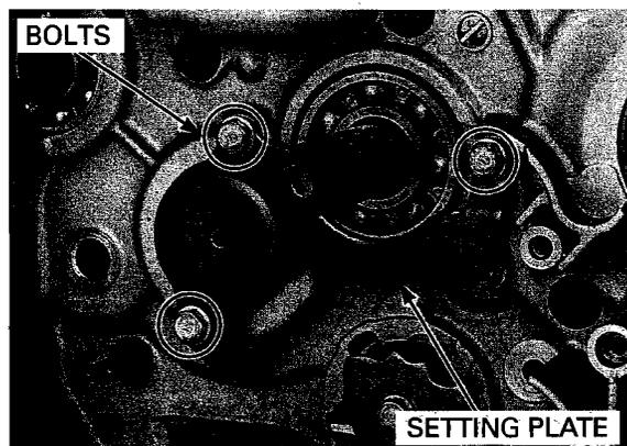
Loosen and remove the 6 mm and 8 mm bolts in a crisscross pattern in several steps.
