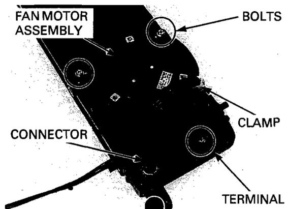
Remove the nut and cooling fan.
