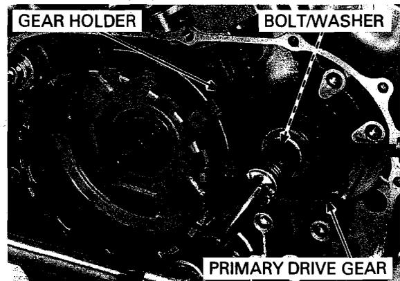
Remove the gear holder and temporarily installed parts.
