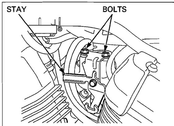
Remove the bolts, intake manifold and O-rings.
