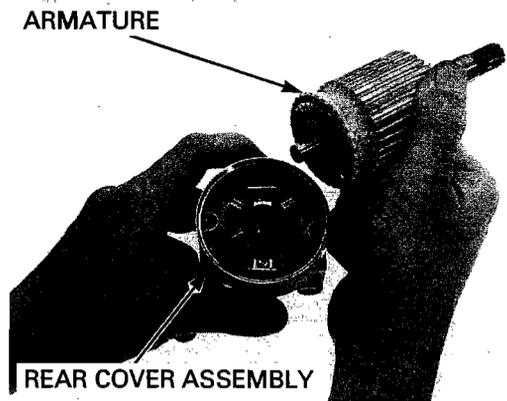
Install a new O-ring to the starter motor case. Install the starter motor case with its groove with the stopper on the rear cover assembly.
