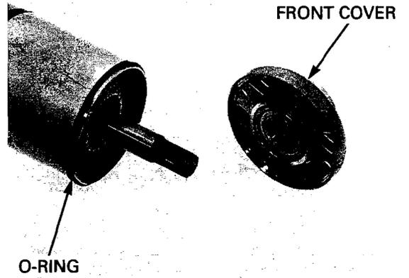
Remove the starter motor case and O-ring.
