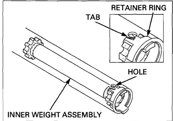
Remove the inner weight assembly from the handlebar.
