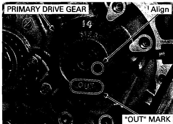
Install the ignition pulse generator rotor, aligning its wide groove with the wide tooth of the crankshaft.
