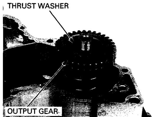
Remove the bushing from the output drive gear shaft.
