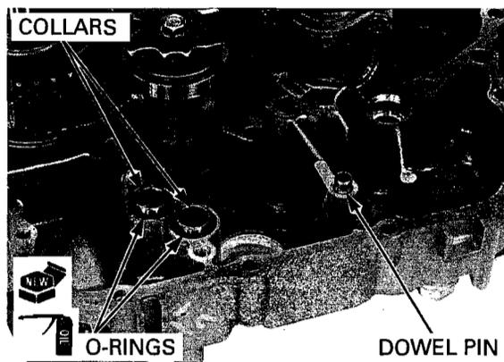
Install the oil pump assembly into the crankcase securely.
