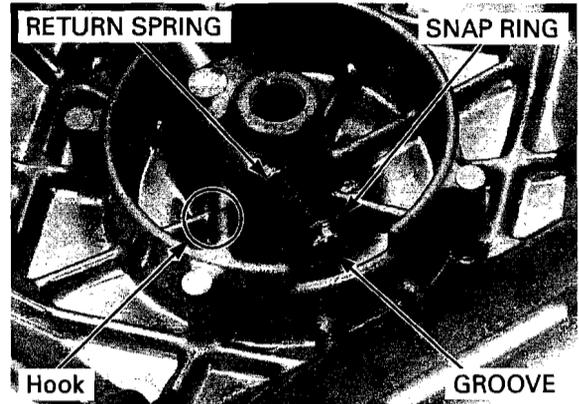
Install the clutch lifter piece, aligning the piece end with the groove in the clutch lifter arm by turning the clutch lifter arm clockwise.
