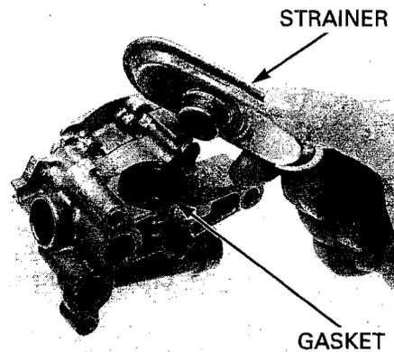
Remove the assembly bolts and pump body from the pump cover.
