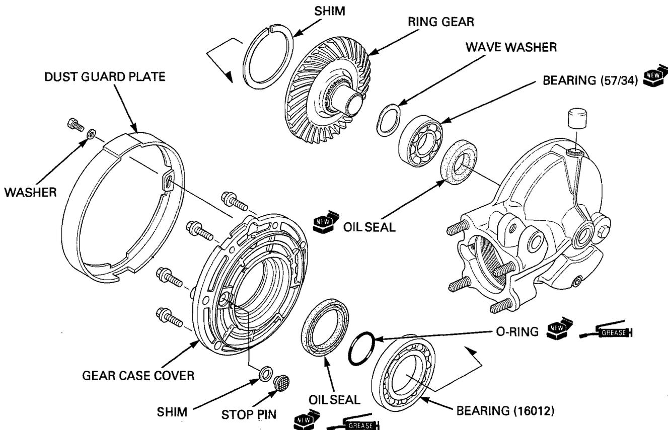
Install the shim onto the ring gear. Support the bearing inner race with the special tool and press the ring gear into the bearing using a hydraulic press.
