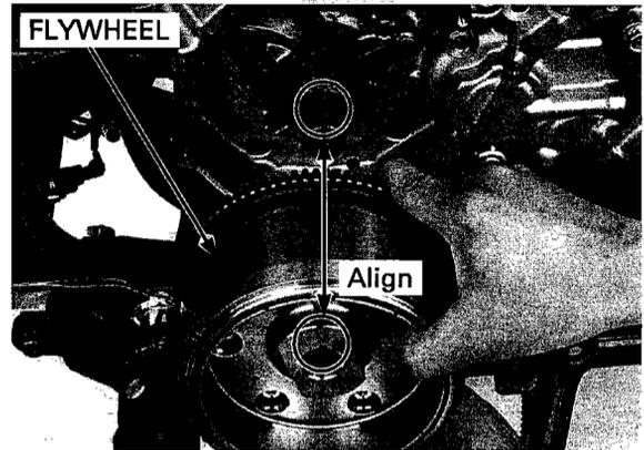
Hold the flywheel using a special tool.
