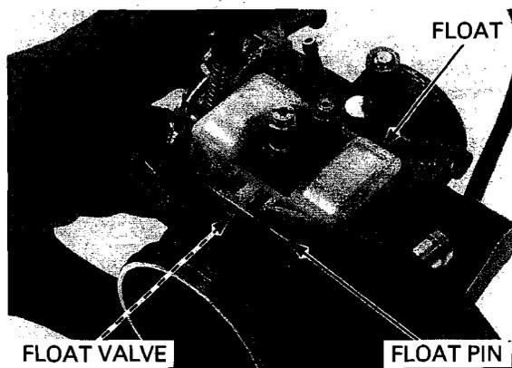
Check the float valve and valve seat for scoring, scratches, clogs or damage.
