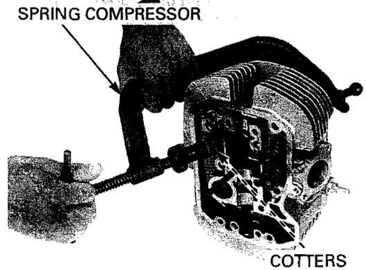
Support the cylinder head so the valve heads will not contact anything and possibly get damaged.
