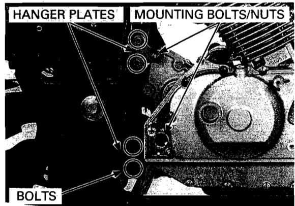
Remove the rear engine mounting bolts.
