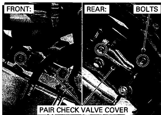
Remove the PAIR check valve from the cylinder head cover.
