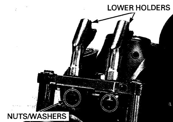
Place the handlebar on the lower holders aligning the punch mark on the handlebar with the top surface of the lower holders. Install the upper holders with its punch mark facing forward.
