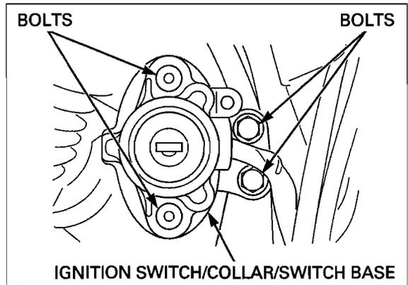
Install the switch base, ignition switch and collar to the stay.
