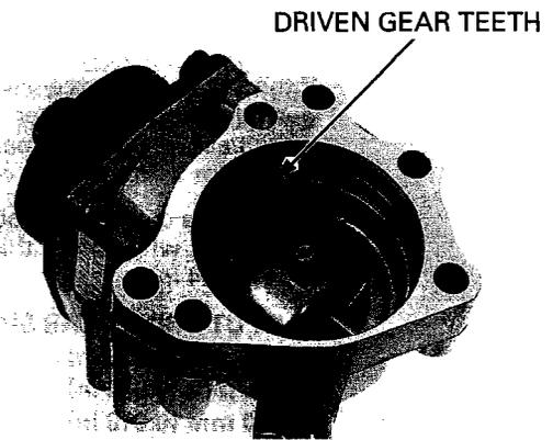
Contact is normal if Prussian Blue is transferred to the approximate center of each tooth and slightly to the toe.
