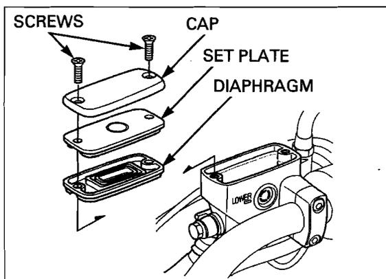
Fill the reservoir with DOT 4 brake fluid from a sealed container to the casting ledge.
