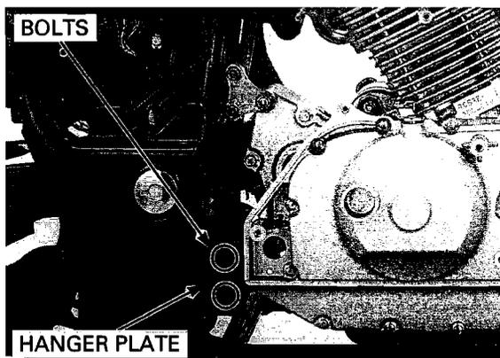
Tighten the left rear upper engine hanger plate bolts to the specified torque.
