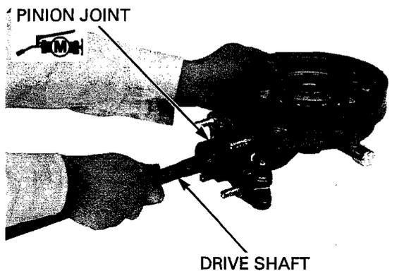
*Make sure the stopper ring is seated properly by pulling on the drive shaft lightly. Be careful not to damage the drive shaft oil seal.*
