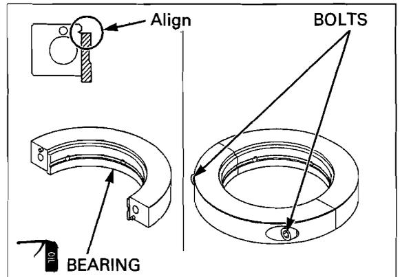
Set the bearings and special tools assembly on inside of the crankcase, fitting the bearing edge in the crankcase main journal.
