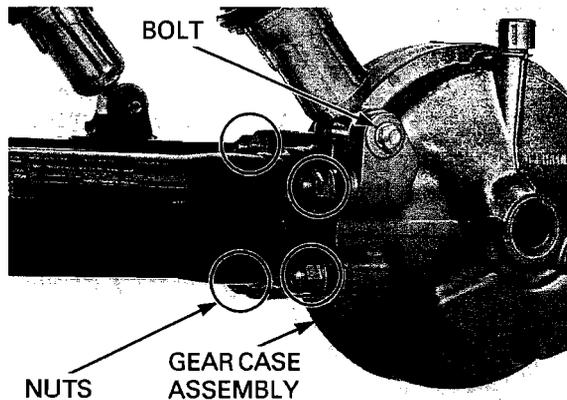
Remove the drive shaft from the final drive gear case assembly by gently turning the drive shaft and pulling it.
