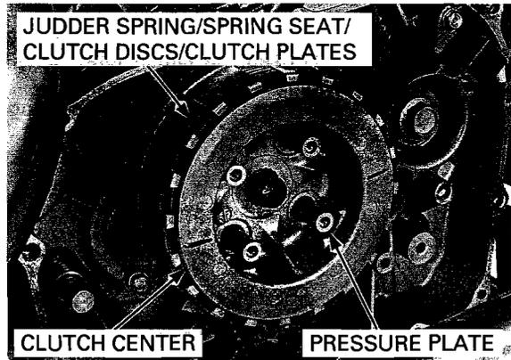
Remove the thrust washer and clutch outer.
