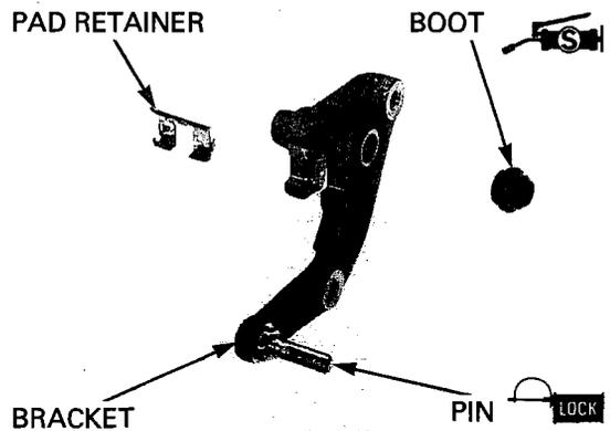
Check the bracket pin boot and replace it if it is hard, deteriorated or damaged.
