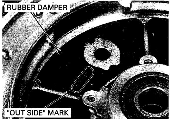
*Install the stopper plate with the "OUT SIDE" mark facing up.*
