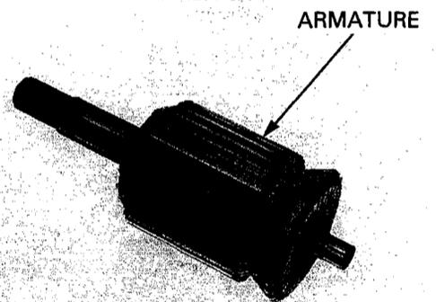
Check for continuity between pairs of commutator bars. There should be continuity.
