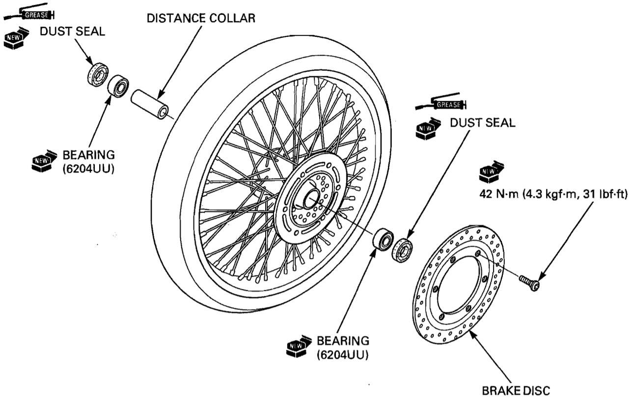
Drive in a new left bearing squarely with the marked side facing up until it is fully seated.
