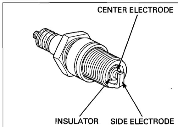
Check the spark plug gap between the center and side electrodes with a feeler gauge.
