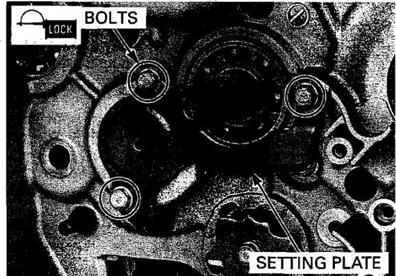
Install and tighten the bolt with the washer by holding the output driven gear shaft using the special tools.
