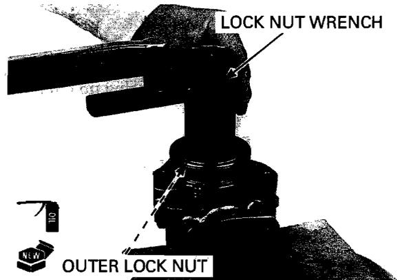
Apply engine oil to the threads and seating surface of a new bearing inner race lock nut and tighten it to the specified torque using the special tools.
