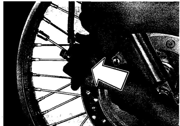
Remove the pad pin plug and loosen the pad pin.
