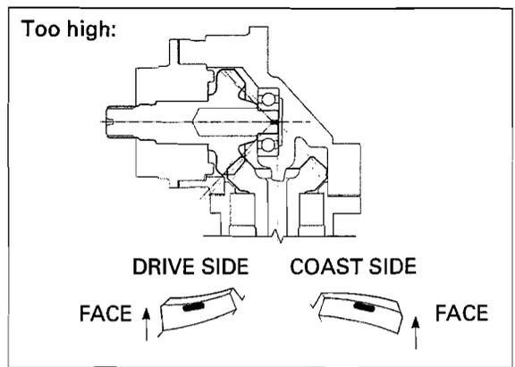
Replace the shim with a thicker one if the contact pattern is too low, toward the flank.
