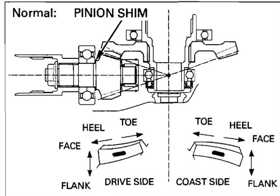
Replace the pinion gear shim with a thicker one if the contact pattern is too high, toward the face.
