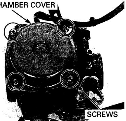
Remove the vacuum chamber cover, compression spring and diaphragm/vacuum piston from the carburetor body.
