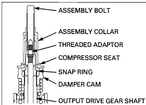
Remove the snap ring, special tools, damper cam and spring from the drive gear shaft.
