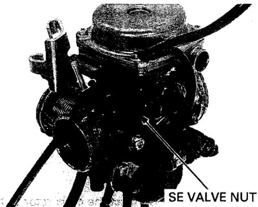
Connect the fuel and PAIR control valve vacuum hoses.
