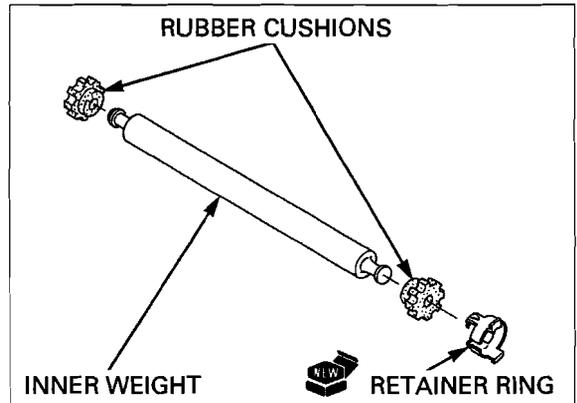
Insert the inner weight assembly into the handlebar by hooking the retainer ring tabs with the holes in the handlebar.
