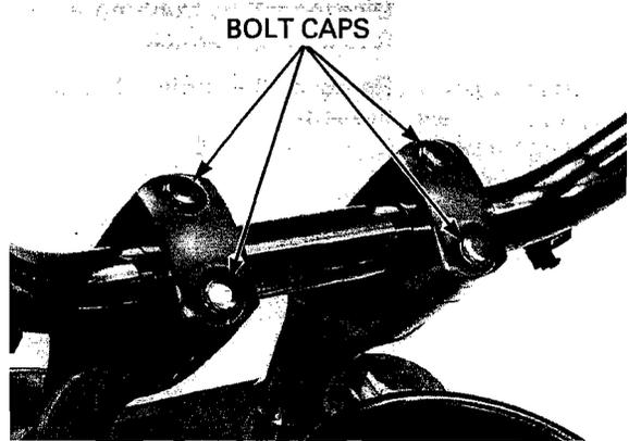
Remove the bolts, upper holders and handlebar.
