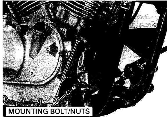
Tighten the rear lower, then rear upper engine mounting nuts to the specified torque.
