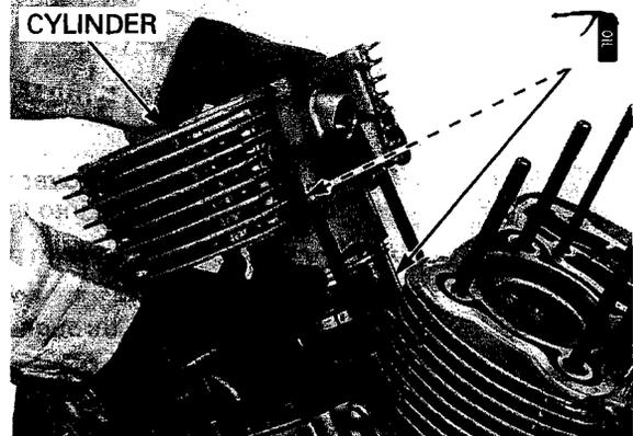
Slide the joint collar into the hole in the cylinder and connect it.
