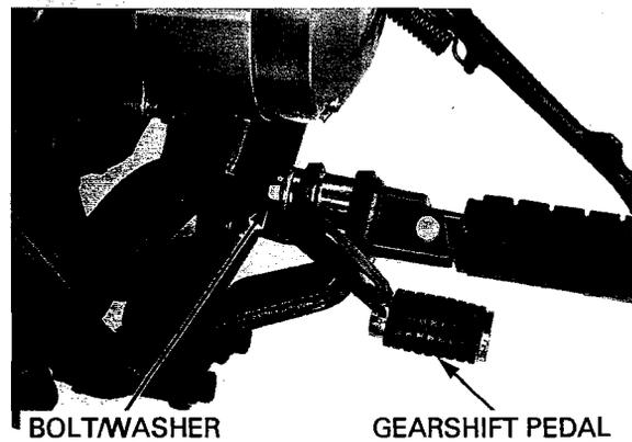
Remove the pivot collar and dust seals from the gearshift pedal.
