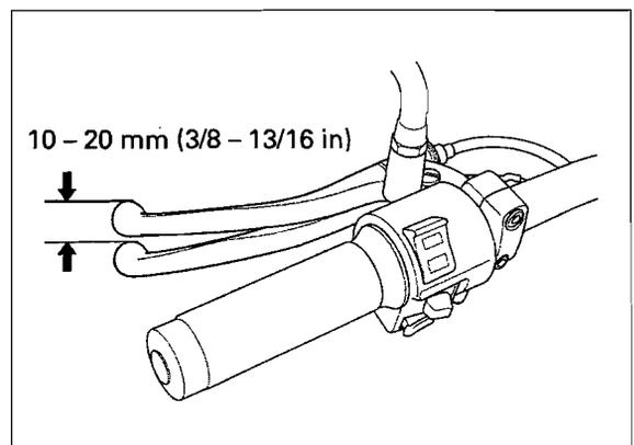
*The adjuster may be damaged if it is positioned too far out, leaving minimal thread engagement.*
