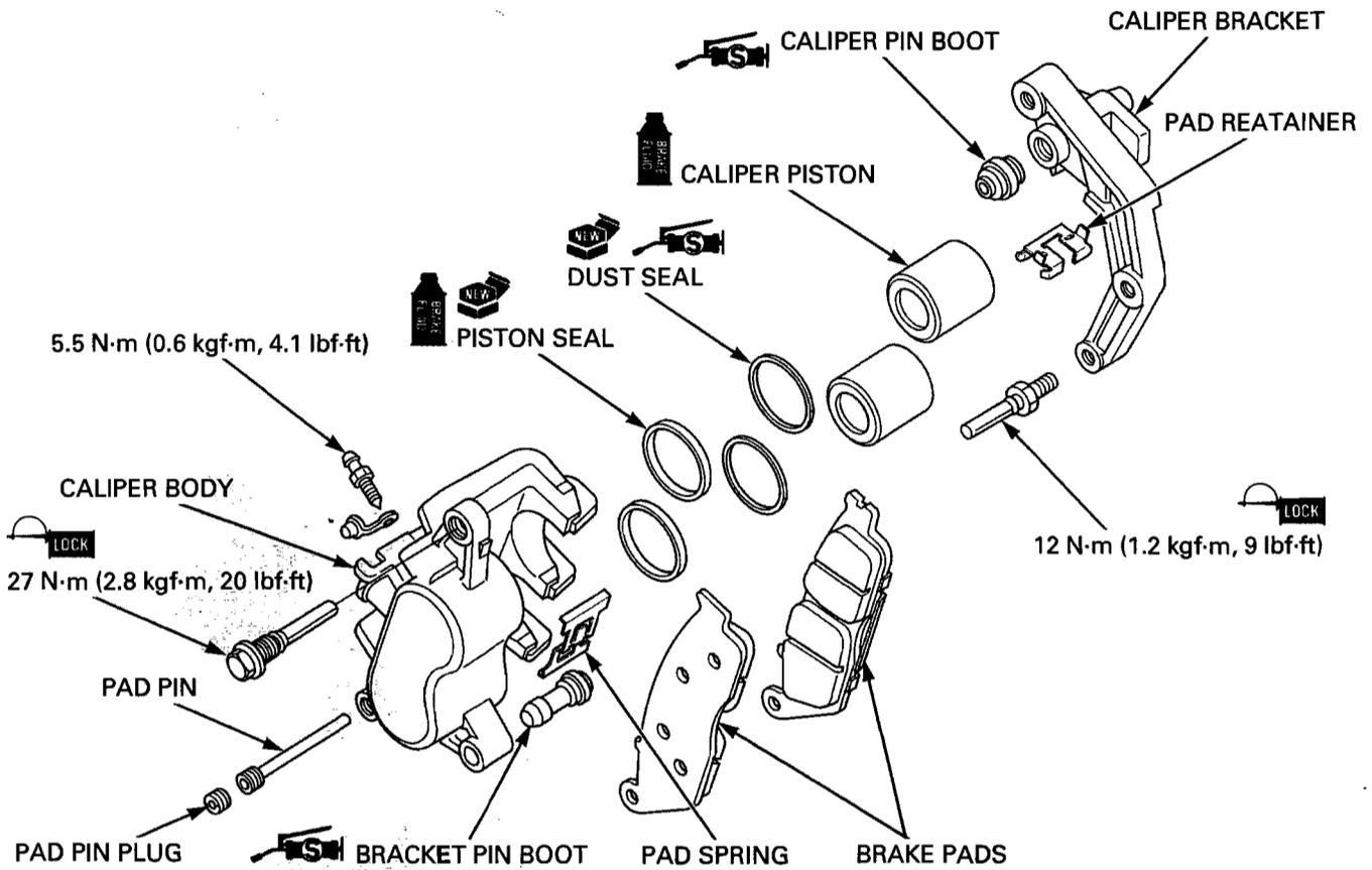
Coat new piston seals with clean brake fluid, new dust seals with silicone grease and install them into the seal grooves in the caliper.
