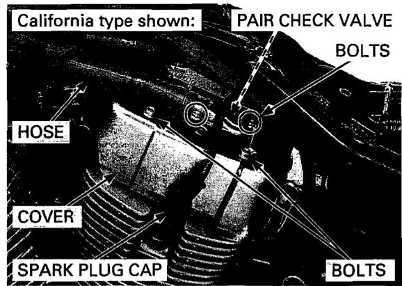
Disconnect the crankcase breather hose from the cylinder head cover.
