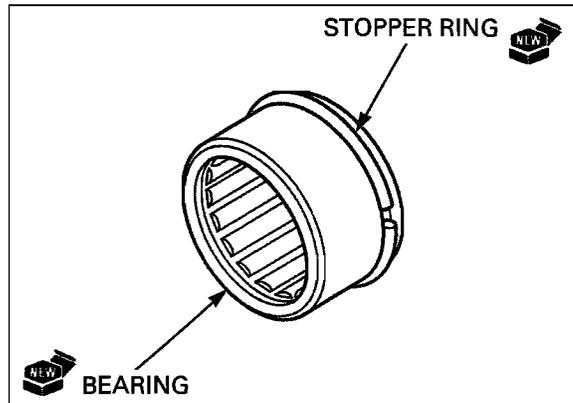
Place the needle bearing in a freezer.
