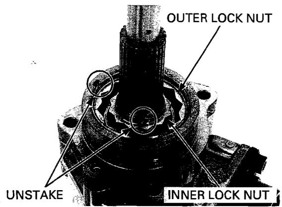
Remove the bearing inner race lock nut using the special tools.
