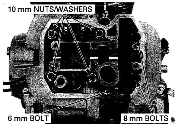
Remove the gasket and dowel pins.
